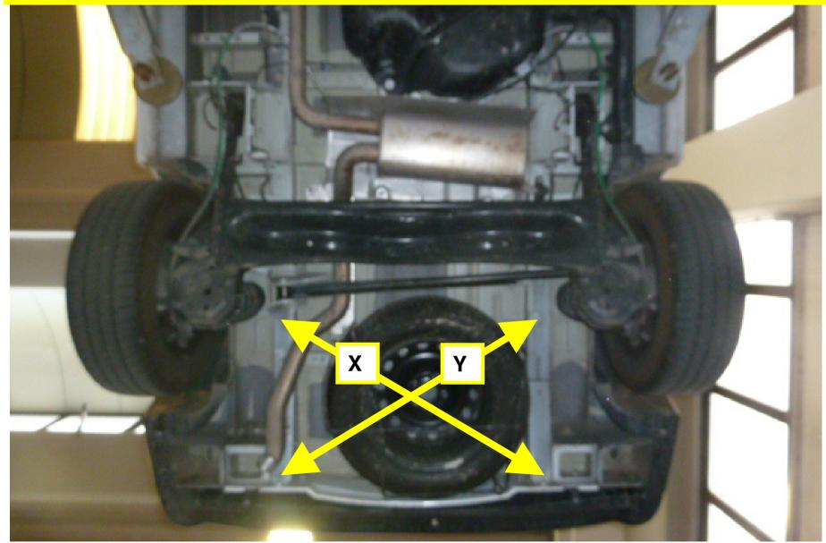
"X" Measures a distance of: 1011mm "Y" Measures a distance of: 1011mm
