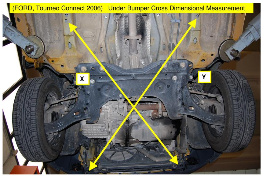
"X" Measures a distance of: ( 1508 )mm "Y" Measures a distance of: ( 1503 )mm
