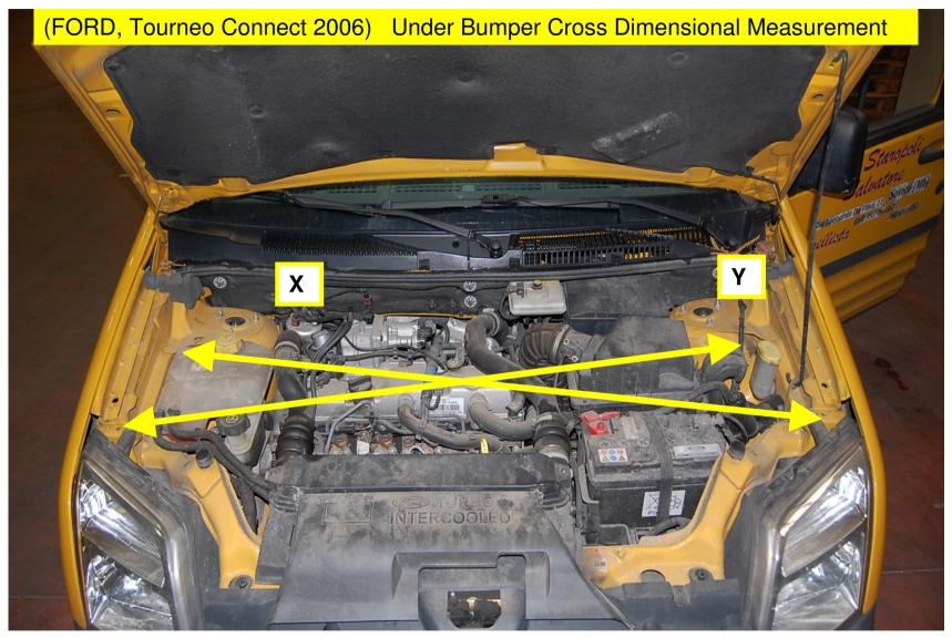
"X" Measures a distance of: ( 1337 )mm "Y" Measures a distance of: ( 1345 )mm
